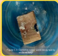
Figure C.3: Control in rubber wood decay test by white rot fungus
