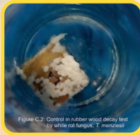
Figure C.2: Control in rubber wood decay test by white rot fungus, T. merizae
