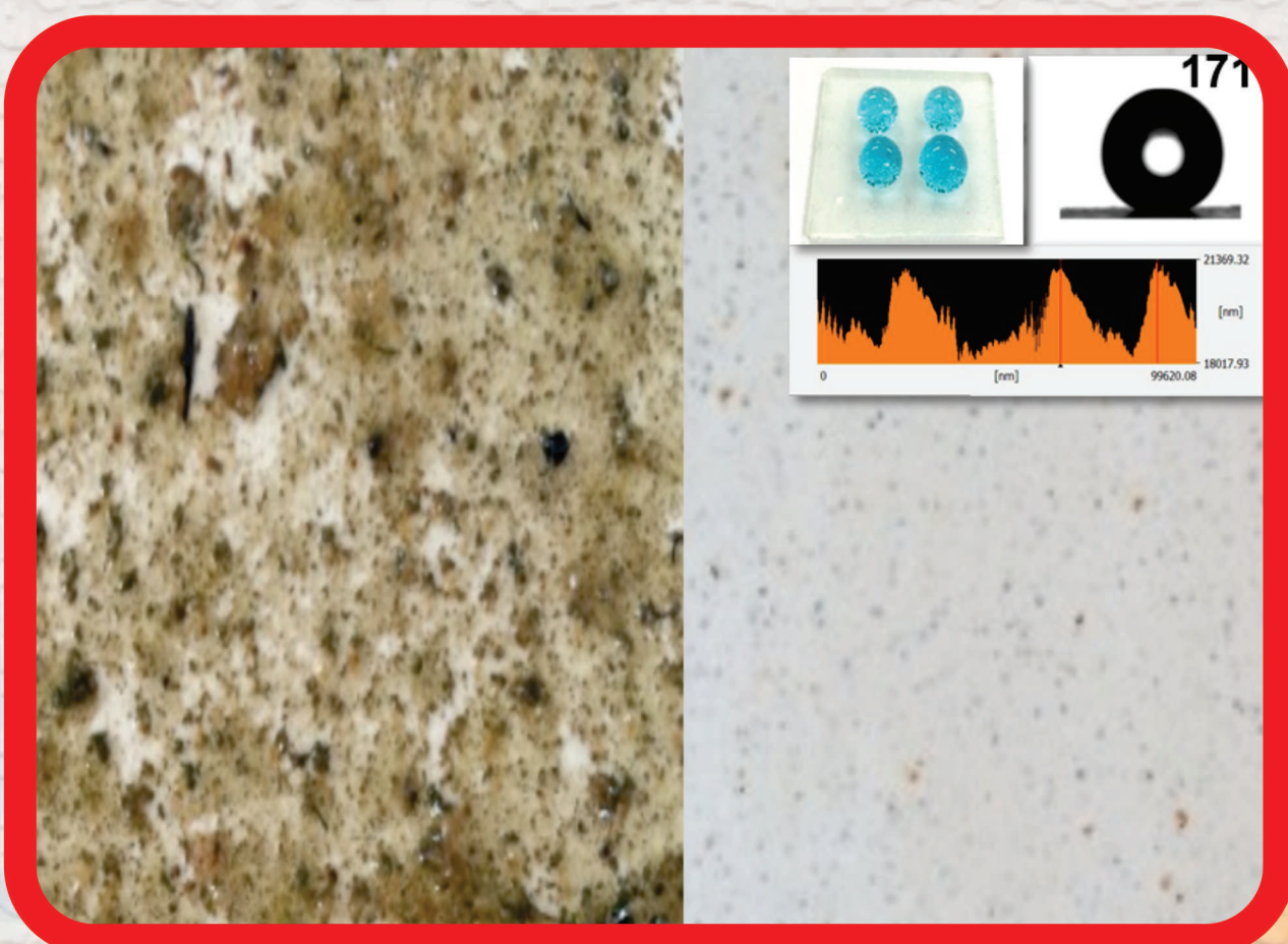
myeco-POFA Shield demonstrates excellent inhibition against fungus growth due to hydrophobic nature of the coating
